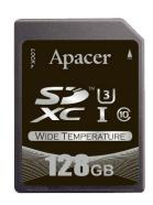
Regarding compatibility, this industrial SD card is compatible with SD Memory Card Specifications, Physical Layer specification, File System Specification and Part 3 Security Specification. Furthermore, the SD card is compatible with SD protocol. With built in ECC, wear-leveling and bad block management, this industrial SD card serves as an ideal portable storage solution.
