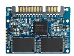
In regard of reliability, the drive comes with various implementations including powerful hardware ECC engine, power saving modes, wear leveling, flash block management, S.M.A.R.T., TRIM, and power failure management.
