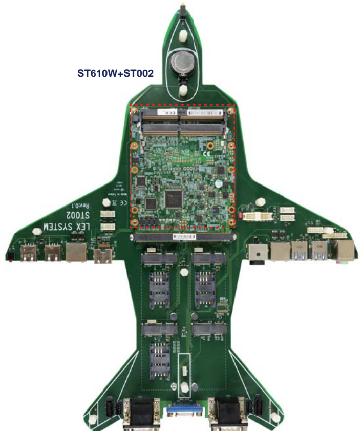
► Evaluation carrier board for ST610W
