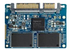
For data efficiency, the internal controlling unit of the SSD is engineered with DRAM for enhanced random performance. In regard of reliability, the drive comes with various implementations including powerful hardware ECC engine, power saving modes, wear leveling, flash block management, S.M.A.R.T., TRIM, and power failure management.
